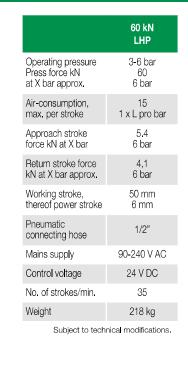
**GECHTER** LHP presses come **INFO** equipped with a ram fine-adjustment mechanism as standard (scaling 0.05 mm)
